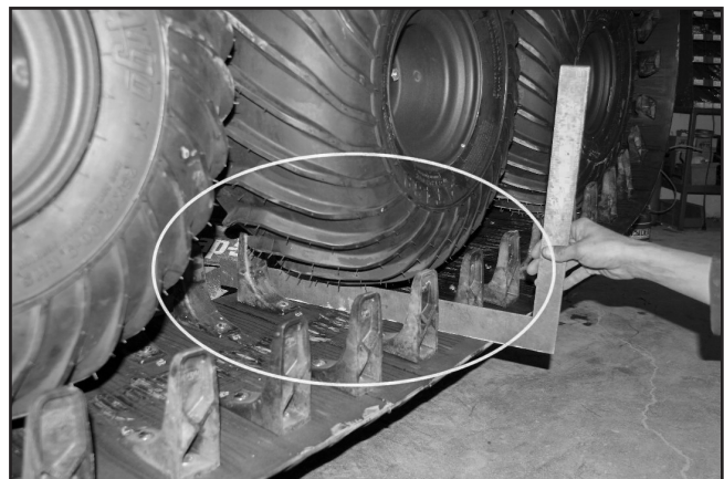
Figure 11-5. Measuring the gap of the mid tires - Avenger.
