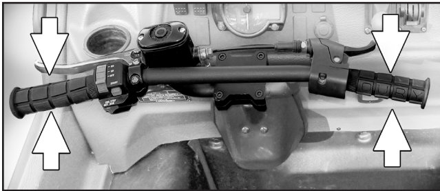
Figure 4-1. Position of moto-cross style steering bar in straight ahead operation.
