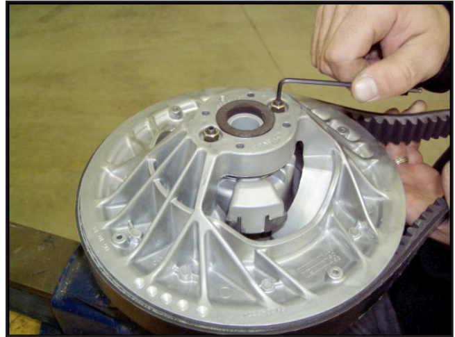
Figure 7-2b. Turn the adjustment set screw.
