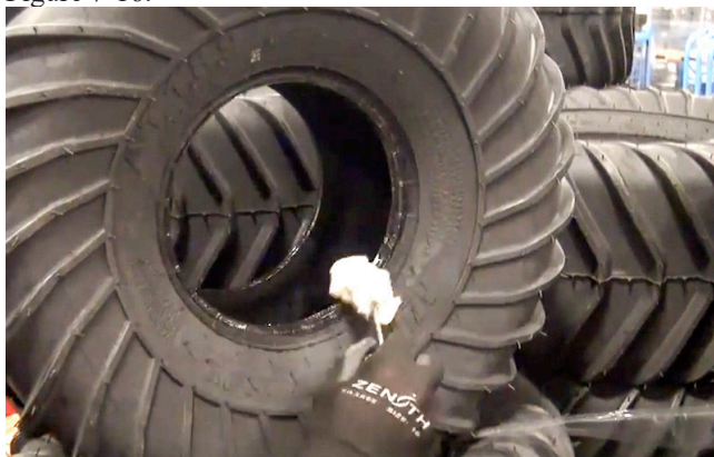
Figure 7-16. Apply tire bead lube.
