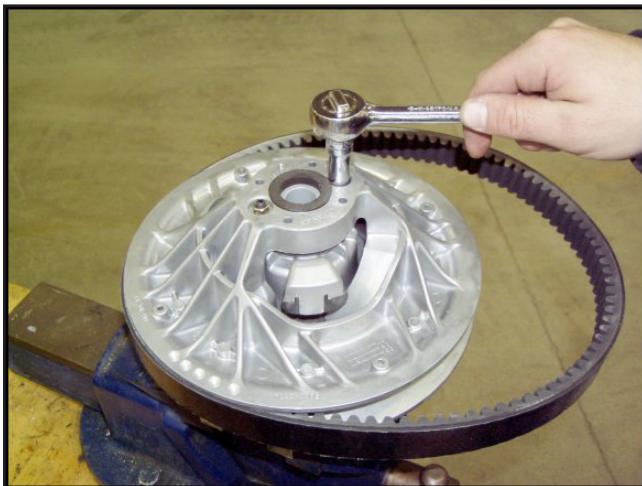
Figure 7-2a. Loosen jam nuts.
