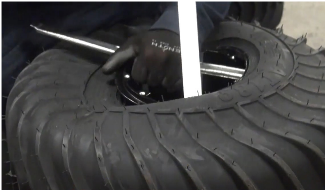
Figure 7-20. Turn rim over and spoon tire onto lip of opposite side.
