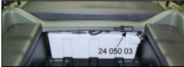
Figure 6-6. Avenger EFI fuel filter location.
