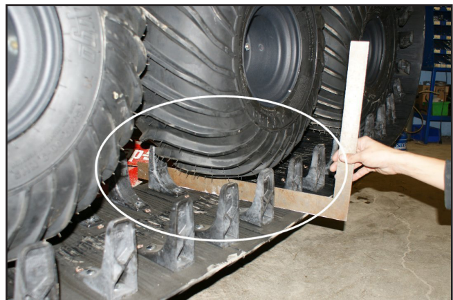
Figure 11-12. Measuring the gap of the mid tires - Avenger.
