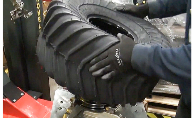
Figure 7-17. Install tire to rim.
