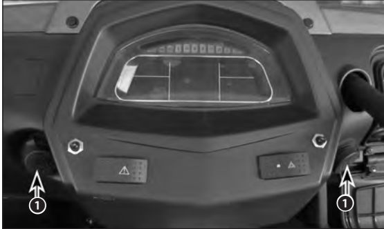
1. 12V DC outlets
