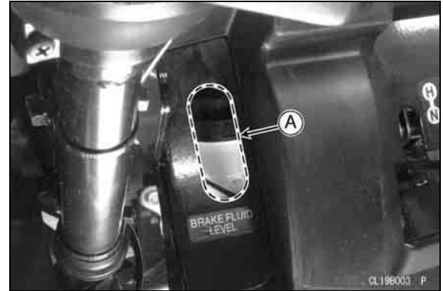
A. Inspection Hole
