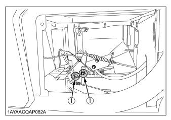
(1) Differential lock pedal (spray type grease)
