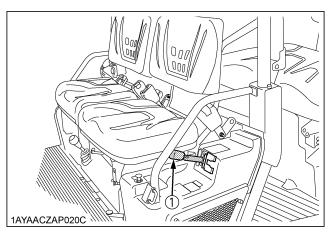
(1) Hydraulic lift cylinder lever
