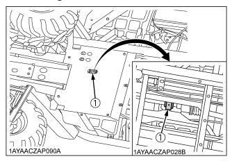
(1) DT shaft bearing (Grease fitting)
