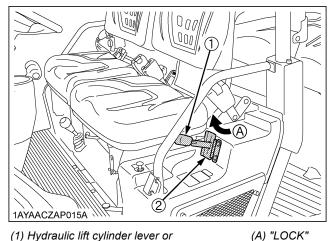
(1) Hydraulic lift cylinder lever or Hydraulic outlet lever (if equipped)
