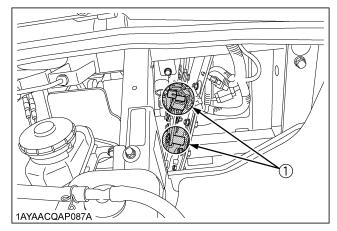
(1) Parking brake lever (spray type grease)
