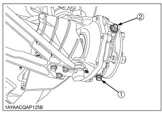
(1) Drain plug (2) Filling plug
