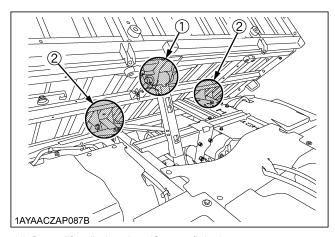
(1) Cargo lift cylinder pivot (Grease fitting)
