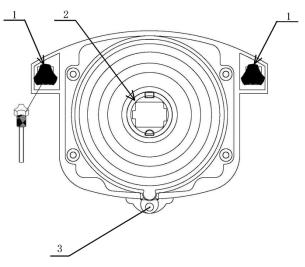
1. To lower headlight brightness cut-off line, turn adjusting bolt (1) counterclockwise. And to raise brightness cut-off line, turn the bolt
