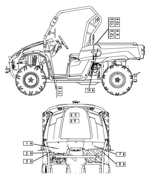
**NOTE:** Warning decals have been placed on the vehicle for your protection. Read and follow the instructions on each decal carefully. In the event any decal becomes illegible or comes off, contact your dealer for a replacement. **Attention:** There is a risk of fire from driving the vehicle on the ground where grass has dried up or parking the vehicle on such surface while the engine is hot.
