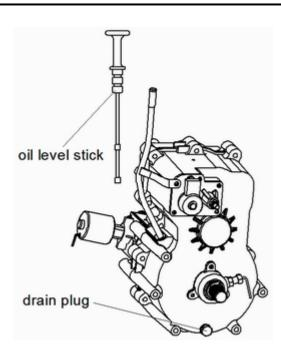
The oil level stick of the transmission is located on the left side of the machine.
