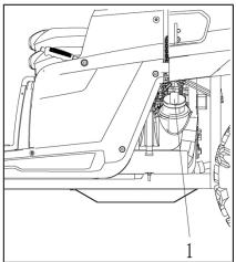
1.Fuel tank cap Remove the fuel tank cap by turning it counterclockwise.
