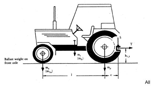
tractors with a loaded mass exceeding 2,5 tonnes must be fitted with a trailer coupling having a ground clearance satisfying one of the following relations:
