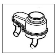
Insufficient brake fluid may let air enter the brake system, possibly causing the brakes to become ineffective. Before riding, check that the brake fluid is above the minimum level mark and replenish if necessary. A low brake fluid level may indicate worn brake pads and/or brake system leakage. If the brake fluid level is low, be sure
