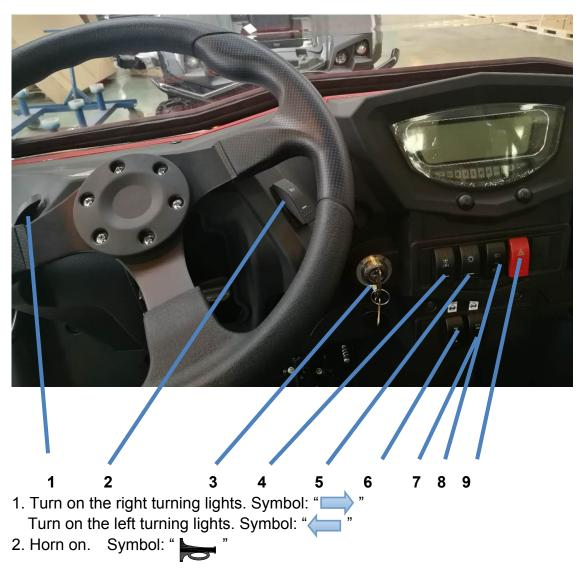
3. Main Switch. This key switch must be turned clockwise to the "on" position to start the engine.
