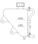
As coolant operating temperature increases, the expanding (heated) excess coolant is forced out of the radiator past the pressure cap and into the recovery bottle. As engine coolant temperature decreases, the contracting (cooled) coolant is drawn back up from the tank past the pressure cap and into the radiator.
