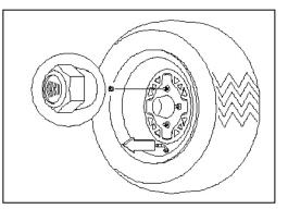
Tapered nuts: install with tapered side against wheel
